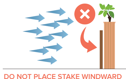
Fig B - Incorrect installation
